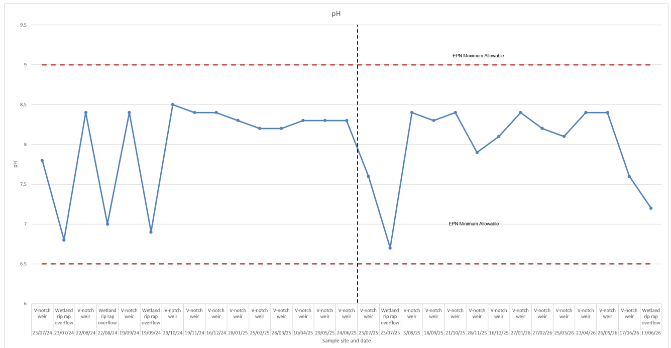
Figure 13 pH - Bypass Creek V-notch weir and Wetland Rip Rap Overflow surface water sampling sites
